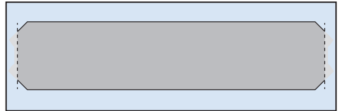
8) Edges cut and burs on sides are "stripped".
