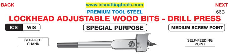
Straight Shank Lockhead Adjustable Wood Bits are designed for drilling in wood using a portable electric drill or drill press. Blade can be adjusted to desired diameter. Does the job of up to 35 different size drills. They are also referred to as Machine Drive Expansive Wood Bits.
