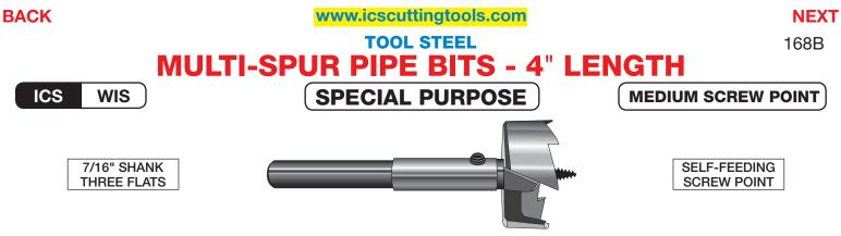
Multi-Spur Pipe Bits are made of special tool steel. Beveled saw teeth allow smooth boring of holes. Inside cutter pushes chips to rear of bit, allowing deep holes to be bored without clogging. Ideal for plumbing and electrical work. They are sometimes referred to as Self-Feed Bits or Saw Tooth Bits. Replacement pilot drills listed below.
