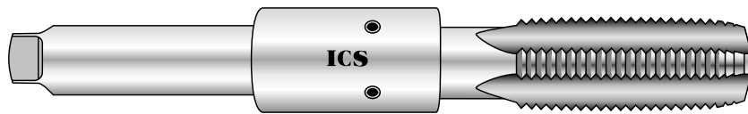
ILLUSTRATION OF 1-3/8 - 6 TAP WITH CUSTOM TAP EXTENSION
