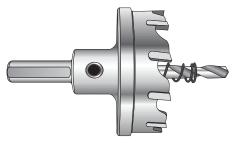
Carbide Tipped Fractional and Metric Hole Cutters are designed for cutting steel plate, stainless steel, galvanized iron, fiberglass, aluminum, and copper up to 3/16" thick. Built-in safety stopper prevents over penetration. Ejector spring ejects slug to save production time. The center drill is a Titanium Nitride coated 135° split point drill. Used by electricians, plumbers, auto and truck repairmen, and general contractors. Outlasts hole saws 5 to 1.
