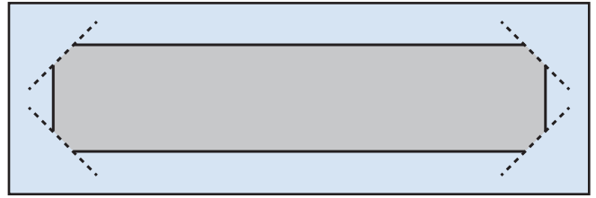
6) Edges and sides are ground.
