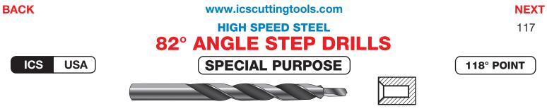
High Speed Steel 82° Angle Step Drills are designed for drilling and countersinking 82° flat head machine screw clearance holes in one operation, saving machine time and reducing set up time. They can be resharpened or modified for a special length of step and are available in jobber length or taper length drill styles.
