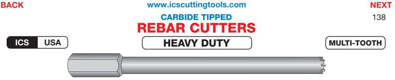
Carbide Tipped Rebar Cutters are designed with a multi-tooth cutter head for drilling through concrete and embedded rebar or wire mesh. Use either water or cutting oil for lubrication and cooling. They can be used in any 1/2" rotary drill with a 3-jawed chuck or directly into SDS, Spline Drive, or SDS-Max Hammer Drills using an ICS rebar cutter adapter.
