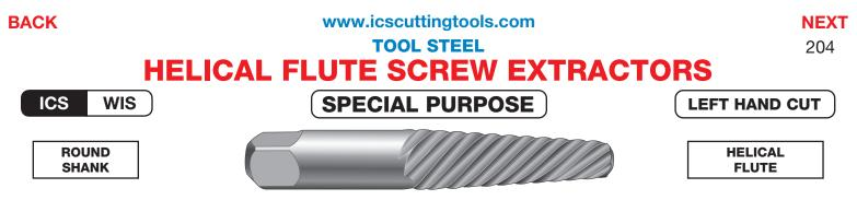
Round Shank Helical Flute Screw Extractors are used to remove broken screws, bolts, studs, pipe, and lubrication fittings without damage to the threaded hole. They are designed with a left hand helical flute to firmly grip and remove any right hand threaded screw or bolt from 3/16" to 3-1/2" in size. They can also be used for turning threaded pipe sections. Sizes #1 to #5 have ground center punch points. Meets Government Specs. GGG-E936B.
