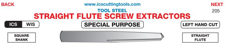
Square Shank Straight Flute Screw Extractors are used to remove broken screws, bolts, studs, pipe, and lubrication fittings without damage to the threaded hole. They are designed with four sharp edges to give a positive gripping action without binding or chewing. They are preferred for soft metals and thin walled parts as they do not expand the part being removed. Meets Government Specs. GGG-E936C.
