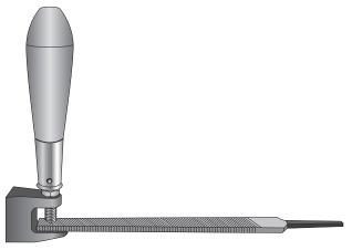
Safety File Handles are designed for machinists doing file work on a lathe. It fits on the point end of the file in an upright position to prevent fingers being under the file during use. Fits all flat or rectangular files. Handle is designed for right hand, left hand, or straight use.
