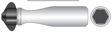
Heavy Duty Plastic Chainsaw File Handle is adjustable and will hold all chainsaw file sizes. End of handle is formed for spark plug removal and installation. Proper guide sharpening angles of 30° and 35° are included on the handle tip.
